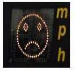
The S.I.D consists of an electronic display which, when sited at the roadside, displays the vehicle speed along with a 'smiley face' for those travelling within the speed limit and a 'grumpy face' for vehicles exceeding the limit.
